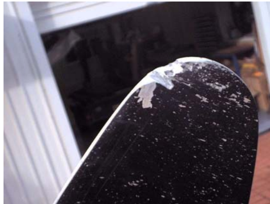
FIGURE 1-13. Propeller Blade Struck by a Foreign Object
