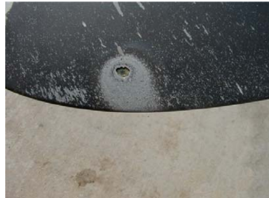
FIGURE 1-12. Lightning Strike on a Composite Surface
